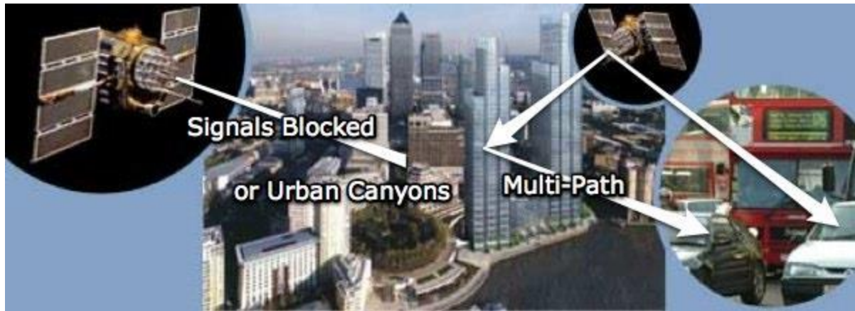
Fig 2: Sources of GPS Signal Error (PocketGPSWorld, 2013)
